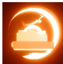
Fig. 3. Silicon droplet on a quasi-single crystal substrate (at a holding time of 1 min)
